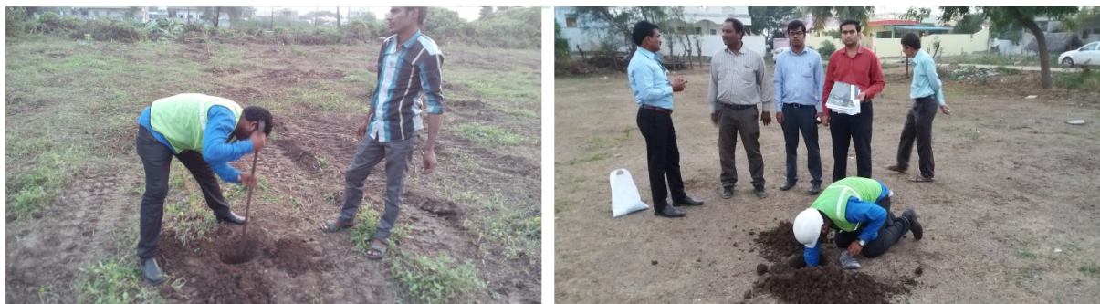
Figure 6-148 Soil sampling near Thullur and Abbarajupalem using Crowbar
