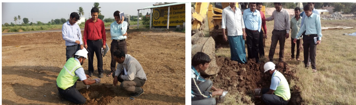
Figure 6-147 Soil sampling near Velagapudi and Malkapuram using Crowbar
