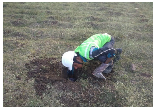
Figure 6-151: Soil sampling near Nidamarru and Penumaka using Crowbar
