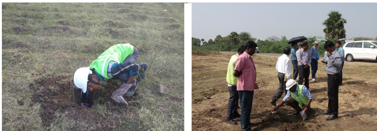
Figure 6-146 Soil sampling near Sakhamuru and Nekkallu using Crowbar
