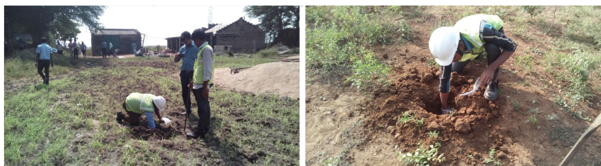
Figure 6-149 Soil sampling near Dondapadu and Rayapudi using Crowbar
